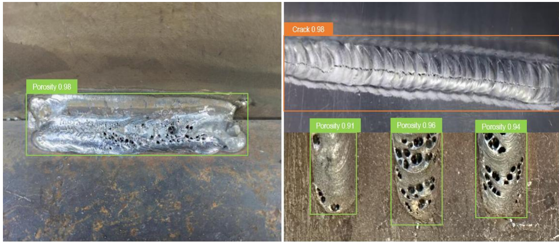
Figure 9. Detective result of YOLOv12 (PConv Based) for welding defect detection.
