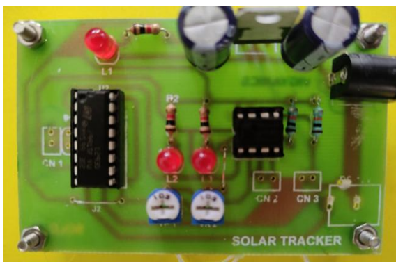
Fig 5. Automatic Solar Tracking System
