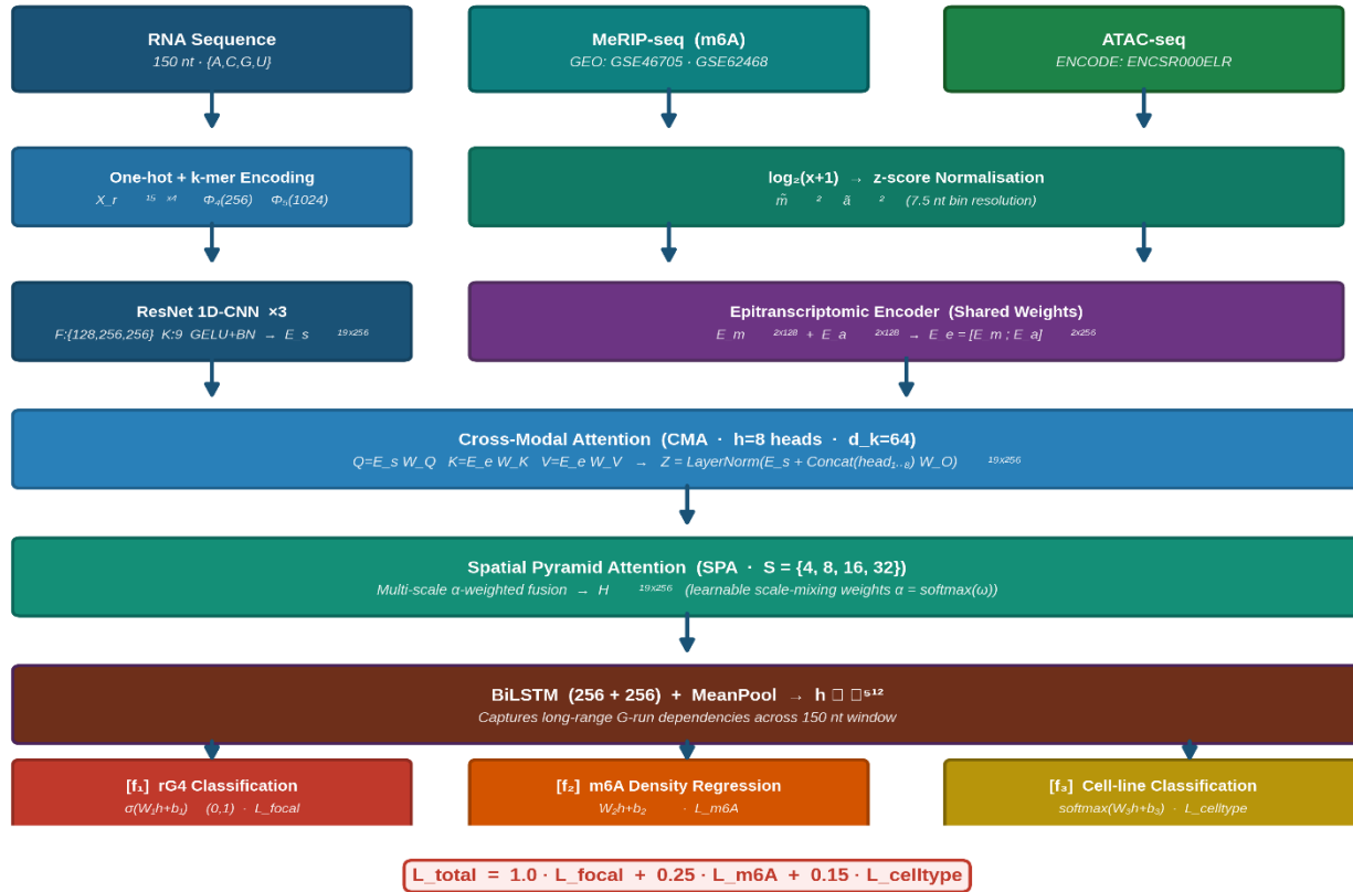
Figure 1. EpiRG4Net system architecture: from multi-modal inputs (RNA sequence + MeRIP-seq m6A + ATAC-seq) through ResNet 1D-CNN encoder, Cross-Modal Attention (CMA), Spatial Pyramid Attention (SPA), BiLSTM, and three-head multi-task output.
