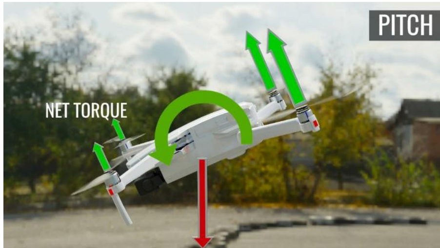
Figure 3.xx: Forces acting on a drone during pitch motion.
