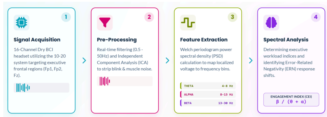
Figure 1. Signal acquisition and processing pipeline of the proposed BCI-EEG model.
