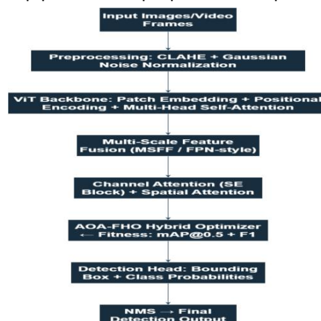
Figure 1. Proposed AOA-FHO ViT framework for multi-object detection.
